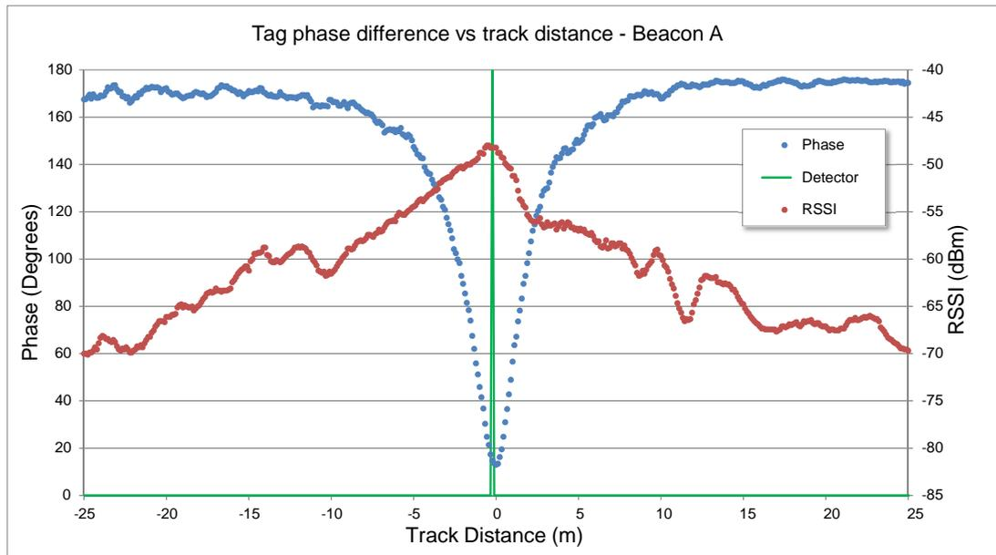
Modern IoT techniques allow trackside beacons to offer positional accuracy similar to track bed beacons for single track sections, without the installation and maintenance challenges of track bed equipment. RSSI is Received Signal Strength Indicator.
