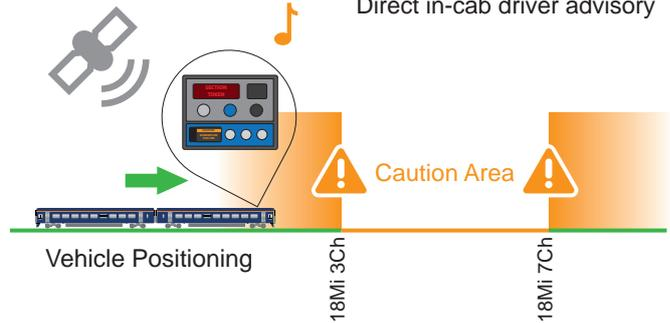
A new digital cautions reminder system allows temporary speed restrictions or other cautionary warnings to be sent directly to in-cab equipment and triggered by train position to give drivers timely caution reminders
